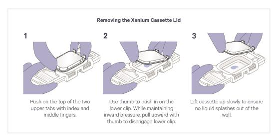
Xenium Cassette Lids are a single use item and should be discarded after each use unless otherwise indicated. PBS-T washes DO NOT require sealing of the cassette with a lid.
